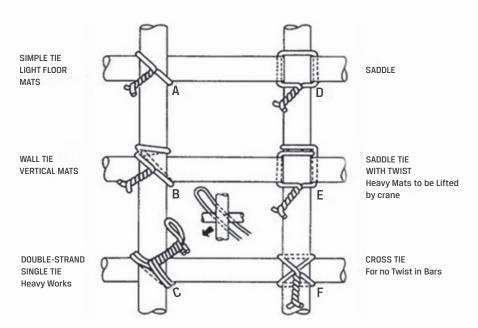
Figure: Six ways to tie rebars.
